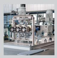
LEWA is the only manufacturer of PTFE-diaphragm pump heads for pressures between 400 bar (5,800 psig) and 1,000 bar (14,500 psig).
