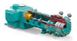
**Piston Compressors:** Howden process gas piston compressors, oil-free or mini-lubricated API618 designs for process applications. Incorporate buffer-purged packing cases and/or double compartment distance pieces, water-cooled cylinders with removable dry liners, and materials engineered to meet any compression application.
